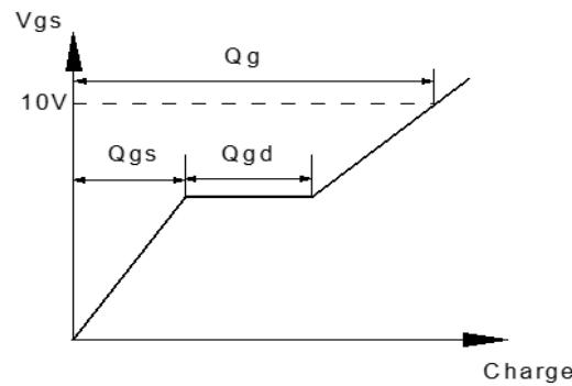
**Figure 1: Gate Charge Test Circuit & Waveform**
