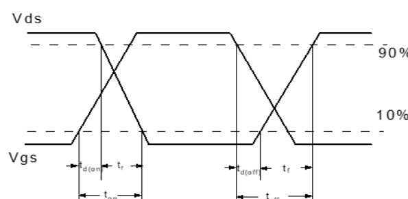
**Figure 2: Resistive Switching Test Circuit & Waveform**
