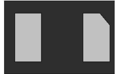
DFN1006-2L (Bottom view)
